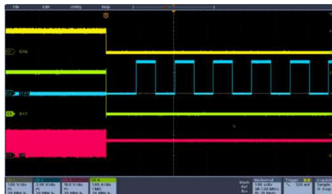
图 10-8 ICHG 短地禁止充电 VBUS = 12V, VBAT = 7.4V, ICHG = 2A
