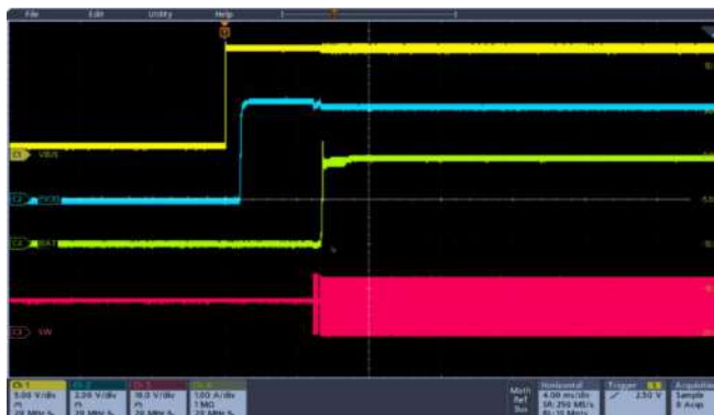
图 10-1 VBUS 启动充电 VBUS = 12V, VBAT = 7.4V, ICHG = 2A
