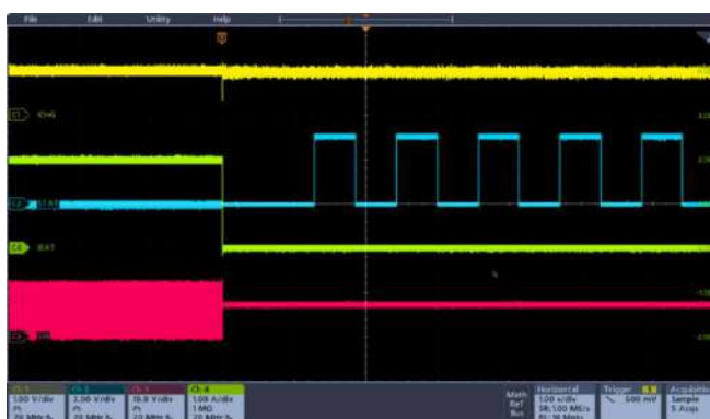
图 10-9 ICHG 开路禁止充电 VBUS = 12V, VBAT = 7.4V, ICHG = 2A
