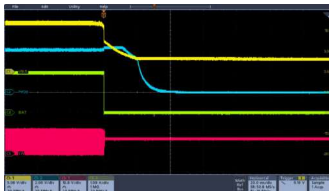
图 10-2 VBUS 掉电 VBUS = 12V, VBAT = 7.4V, ICHG = 2A
