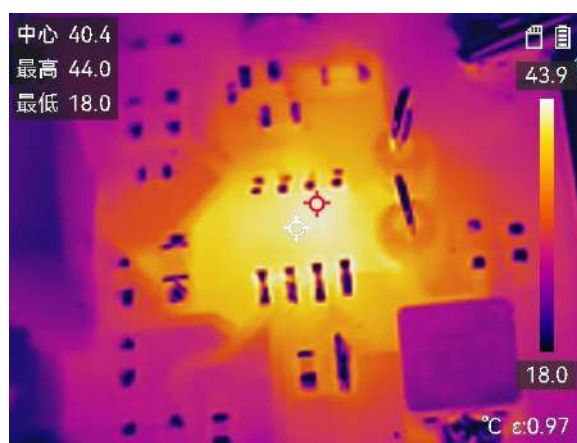
图 10-13 热成像图 (ESOP-8) VBUS = 5V, VBAT = 3.8V, ICHG = 2A
