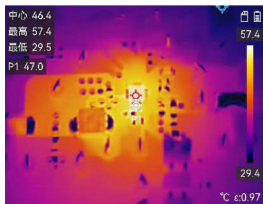
图 10-10 充电时的板级温度 VBUS = 5V, VBAT = 3.8V, ICHG = 2A
